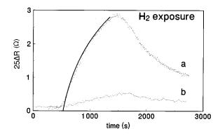
FIG. 1. Resistance changes of Nb films when exposed to  $\rm H_2$  (500–1500 s) and after removal of the gas. Curve a, 40 nm; curve b, 400 nm. Solid line for curve b corresponds to fits to Eq. (3.1).
