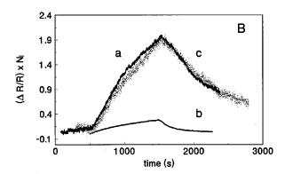
FIG. 2. (a) Resistance changes of Nb and Co films exposed to CO (500–1500 s) and after the removal of the gas. Curve a, 40 nm Nb film; curve b, 10 nm Co film; curve c, 400 nm Nb film. Solid lines for all the curves correspond to curve fitting using Eq. (3.1). (b) Normalized resistance change multiplied by thickness of film ( $N_l$ ) in a number of layers. Curves a, b, and c correspond to the same samples as (a).
