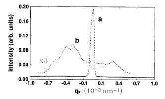
FIG. 4. Transverse scans ("rocking curves") for the Nb (curve a) and Co (curve b) samples.  $q_{zo}$ , as defined in the text, is 0.8535 nm<sup>-1</sup> for Co and 0.9104 nm<sup>-1</sup> for Nb. Note the low specular intensity of the Co sample with respect to the diffuse background.
