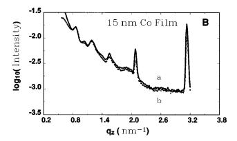
FIG. 3. Longitudinal  $(\theta - 2\theta)$  x-ray reflectivity scans of the (a) 40 nm Nb and (b) 15 nm Co sample. Curve a represents the specular reflectivity and curve b the diffuse near-specular reflectivity. Note the low specular intensity of the Co sample with respect to the diffuse background.
